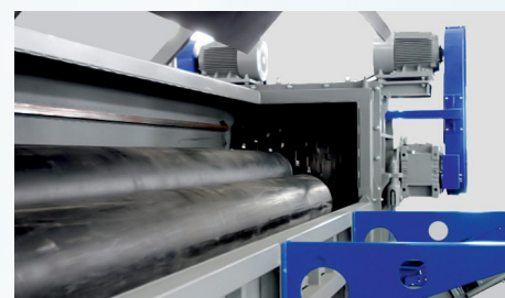
The pipe shredder is equipped with a special feeding trough sized to take pipes of up to 6m length. A powerful hydraulic ram forces the pipes into the rotor.
