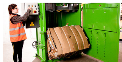
High compaction ratio creates the optimum 250 kg bale
