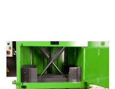
Cross ram and long-stroke cylinder for optimum compression in a small space
